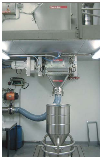
Sack tipping station for breaking up of granules; execution for CIP cleaning
